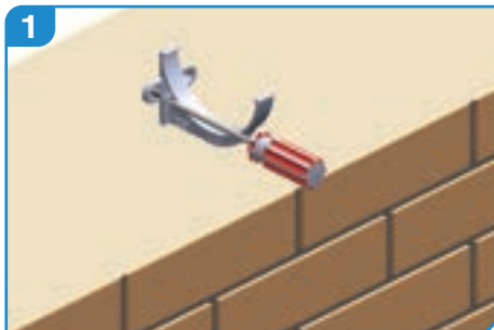
1 Identify the highest and lowest point of the gutter run and install brackets on each end ensuring a minimum fall of 1:600.
