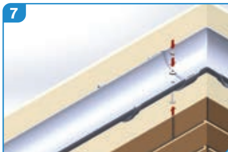
7 Push bolt through the sole of the gutter socket ensuring that the slot is filled with sealant before applying nut and washer, gently tighten. Do not overtighten as this may force the sealant out of the joint.
