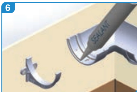
6 Ensure that all fixing surfaces are clean and dry. Apply 2 x 6mm beads of low modulus sealant into the socket end of gutter, place gutter length into sealant/socket.
