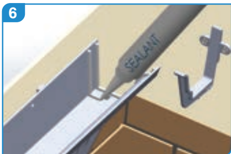
6 Ensure that all fixing surfaces are clean and dry. Apply 2 x 6mm beads of low modulus sealant into the plain end of the gutter, place the spigot end of the gutter length into sealant.
