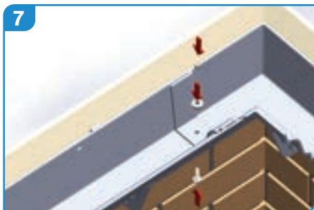
7 Push bolt through the sole of the plain end of the gutter from the underside and position spigot end of gutter directly over joint. Ensure that the slot is filled with sealant before applying nut and washer, gently tighten. Do not overtighten as this may force the sealant out of the joint.
