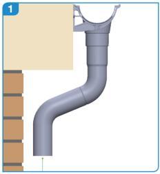
Ensure vertical alignment between drain and gutter outlet.
