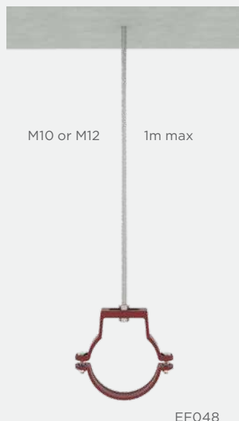
Typical support arrangement for horizontal pipework
