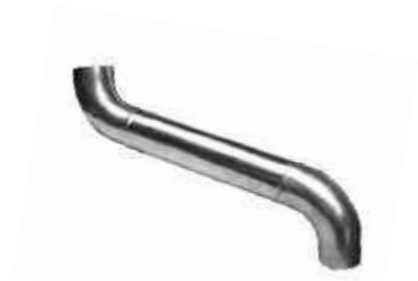
2 72° Bends and 300mm of Downpipe
