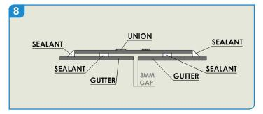
Clean off excess sealant along the edges of the joint. Use the same process for every joint until the work is completed
