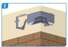
Image 2 shows the bracket for the angle and a bracket to take the gutter length.
