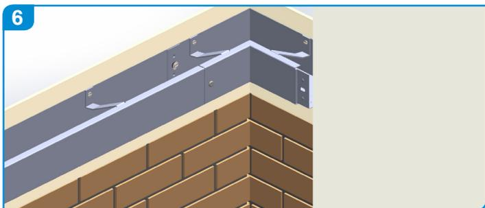
Apply nuts and washers and gently tighten (Do not overtighten as this may force the sealant out of the joint).
