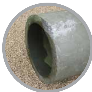
When surface damage prevents a reliable external seal
