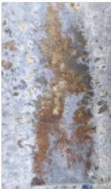
After 6 weeks salt spray test
